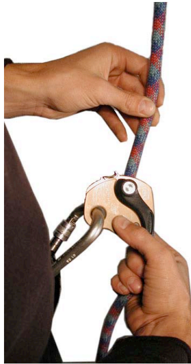
Correct technique for holding the Cinch. Use the left hand to feed rope. Note: hands can be switched.
